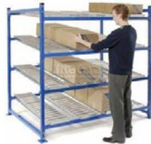
to physically lift and move product to the next operation station, reducing operator motion and improving safety. Gravity flow racking systems also accommodate good visual replenishment. By walking down the backside of the flow rack, it is easy to see which slots are empty or low requiring replenishment to keep assembly work moving.
