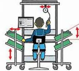
are repetitively moving, retrieving, lifting, twisting, and transferring materials. These areas can be probable points where gravity flow racking applications could be useful to reduce motion keeping production work flowing while improving safety.
